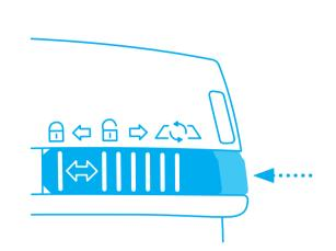
Use the 3-in-1 activator to **lock your cutting tool** after cutting.
