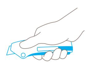
To **engage the blade**, unlock the cutter and squeeze the lever. Now you can cut.
